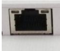
Figure 978: RJ45 LAN Connector
