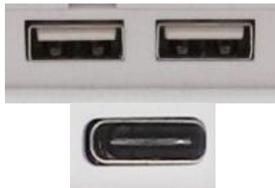
Figure 977: USB HOST and USB TYPE-C Connectors
