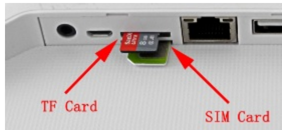
Figure 979: TF Card Slot (upper) and SIM Card Slot (lower)
