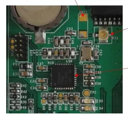
External Zigbee Antenna Connector
