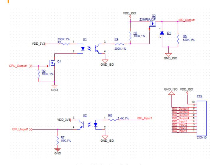
Isolated GPIO reduced schematic
