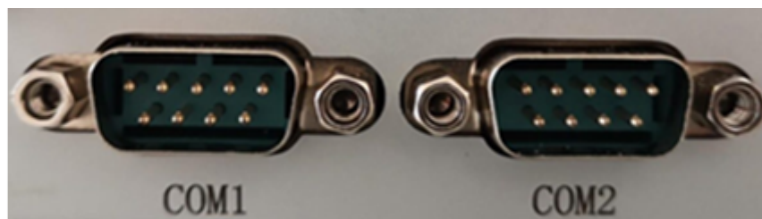
Figure 917: Figure 2: D-Sub (2 x RS232/485)
