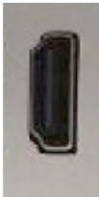
Figure 920: Figure 5: HDMI Connector
