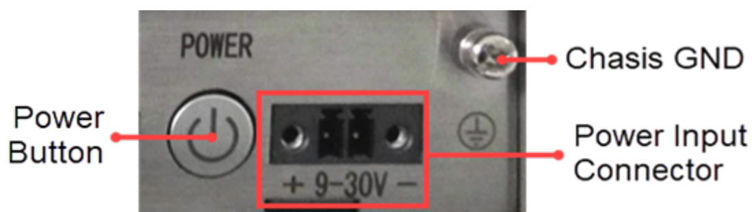
Figure 890: Figure 1: Power Input Section
