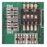
Figure 129: Boot Mode Setup
