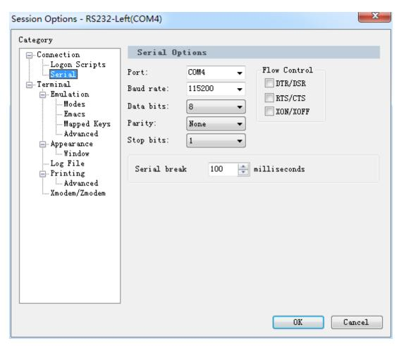
Figure 158: SecureCRT configuration
