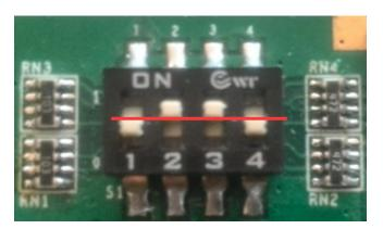
Figure 133: Boot Switch Config
