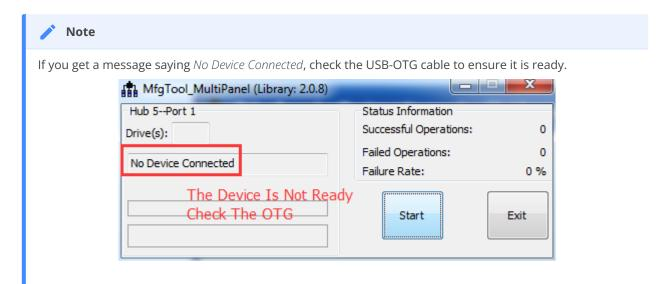
**Figure 136:** The USB-OTG cable is not connected correctly.
