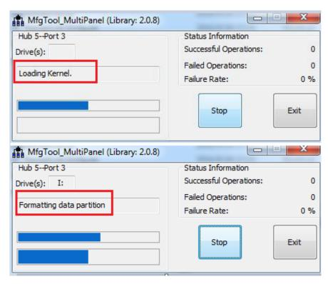
Figure 137: Loading Kernel and Formatting rootfs partition
