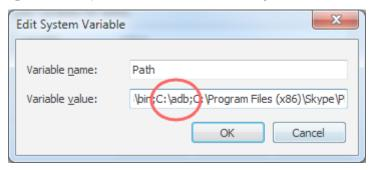
Figure 149: Add path of the ADB directory to the Path system variable
