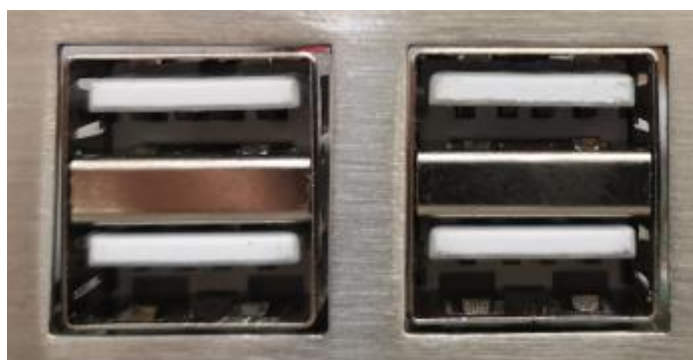
Figure 575: USB 2.0 HOST Connectors
