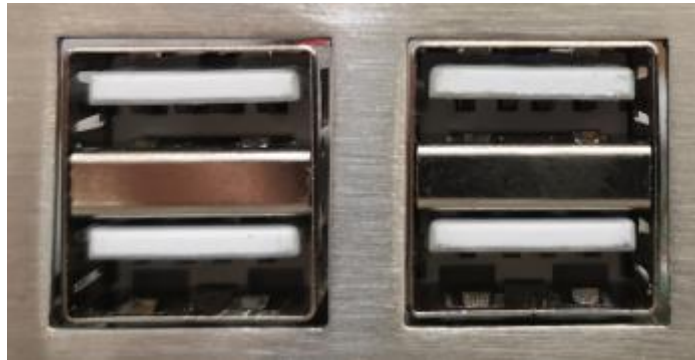
Figure 538: USB 2.0 HOST Connectors
