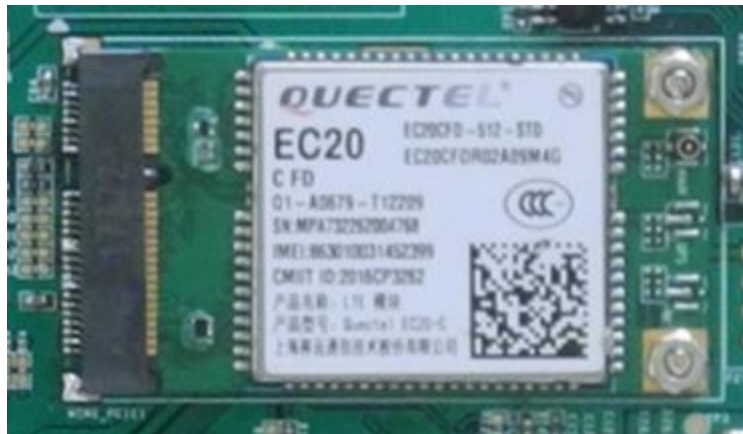
Figure 448: mini-PCIe Connector & 4G Module
