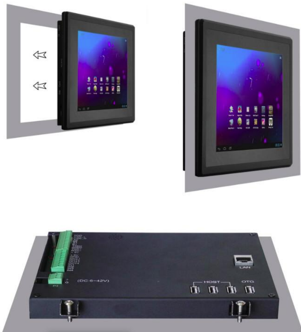
Figure 696: Fixing PPC-A8-101-R industrial PC into panel
