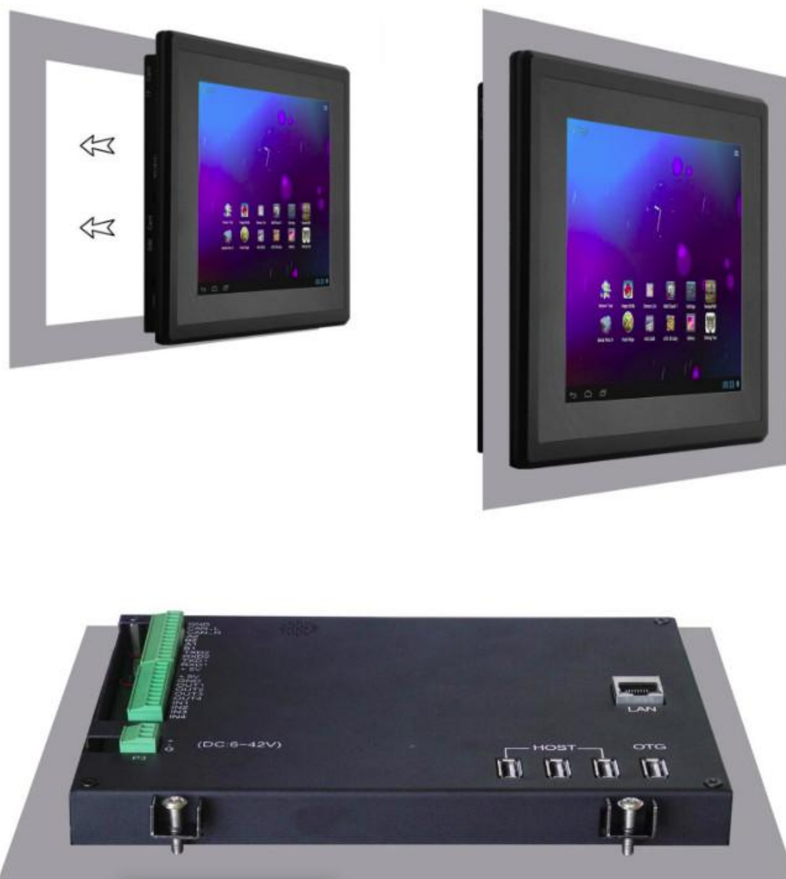
Figure 711: Fixing PPC-A8-070H-C industrial PC into panel
